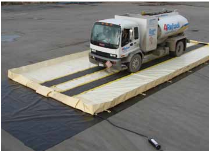
Collapsible hands-free flotation walls allow vehicles to repeatedly enter and exit the berm without manual setup.
