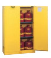
Self-Close This style self-indexes, self-latches and self-closes to automatically shut doors upon release. Mechanism is concealed in the top wall, maximizing available shelf space. Fusible links hold doors open during use. In the event of a fire, fusible links will melt at 165° F (74° C) to automatically close doors.
