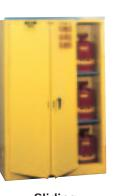
**Sliding** A single bi-fold, sliding door glides smoothly on a spring loaded track for easy, one handed access to cabinet contents. It self-latches and self-closes, and is equipped with a fusible link to hold the door open during use and melts at 165° F (74° C) to automatically close door under fire conditions.
