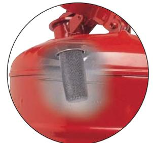
Internal dual-density flame arrester within the fill/pour spout dissipates heat to prevent flashback ignition and guards against the potential for fire and bomb-like explosion. Double mesh construction (a fine mesh screen joined with a coarse mesh screen) protects against fire yet keeps liquids flowing freely for convenient filling and pouring.
